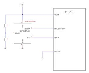
In this case you need a python script that toggles the GPIOx; in this way the module is reset in case it remains stuck for some reason.
