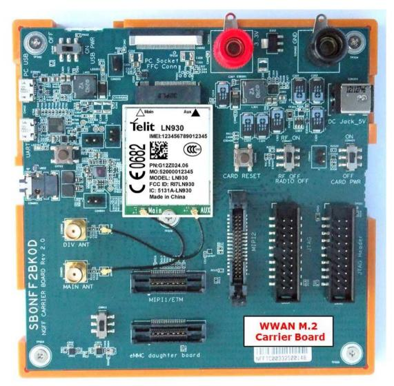
Figure 11 M.2 Carrier Board
