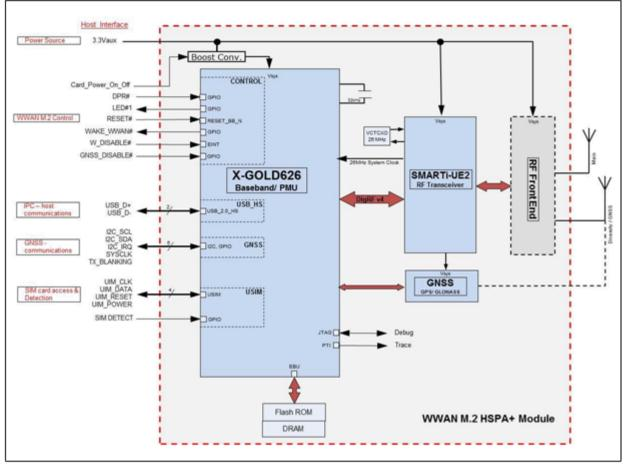
Figure 1 M.2 HSPA+ Block Diagram
