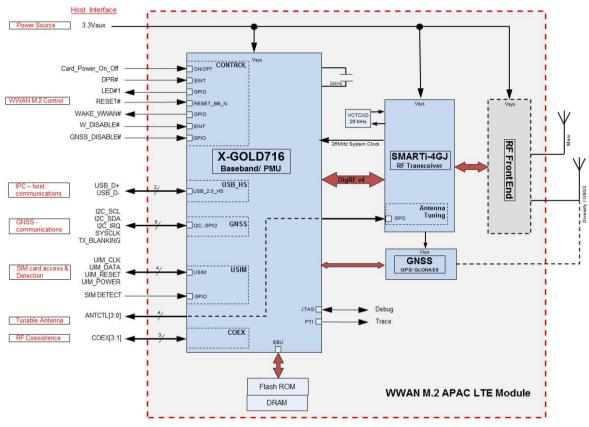
Figure 2 M.2 APAC LTE Module Block Diagram
