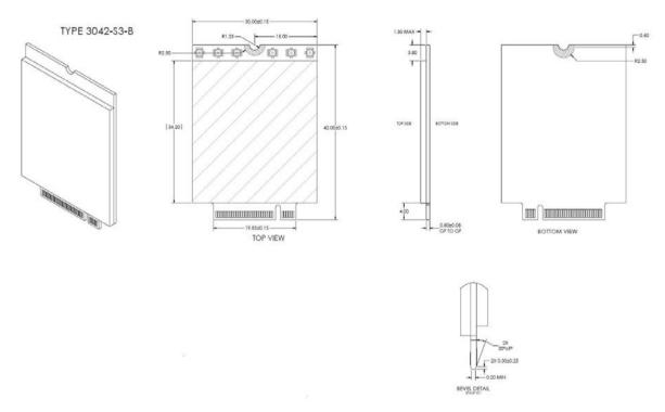
Figure 17 WWAN Card 3042 Mechanical Dimensions
