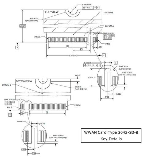
Figure 18 WWAN Card 3042 Slot Key Details
