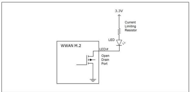
Figure 7 Typical LED Connection
