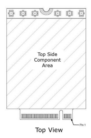
Figure 10 RF Antenna – Coaxial Connector Location
