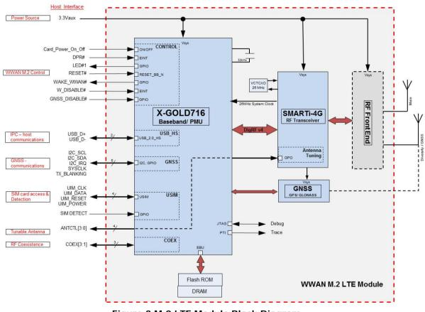
Figure 3 M.2 LTE Module Block Diagram
