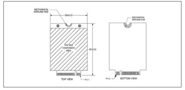
Figure 5 PCI Express M.2 Module Interface
