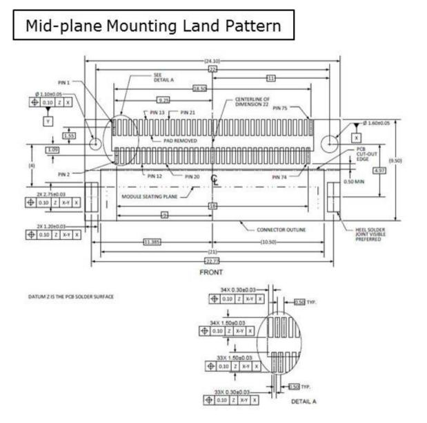
Figure 20 illustrates a typical mid-plane (in-line) land pattern with slot key removed.
