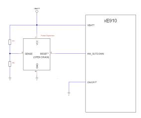
This is just an example: R1 and R2 determine the threshold voltage at which the RESET\* is released, R1 and R2 should be choose in order to have a threshold up to 3.22V.
